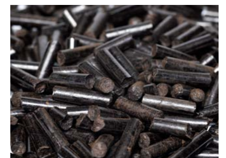
↑ Pellets from torrefied wood
